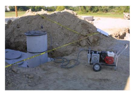
The NPCA standard states: "The recommended vacuum test procedure is to introduce a vacuum of 4 inches of mercury. Hold this pressure for five minutes. During this initial five minutes, there is an allowable pressure equalization loss of up to 1/2 inch of mercury. If the pressure drops, it must be brought back to 4 inches and held for a further five minutes with no pressure drop."
