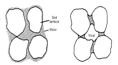
Illustrating the effect of two different water contents on the degree of filling of soil pores. On the left, a saturated condition wherein all pores are filled; and at the right, an unsaturated condition wherein water is retained principally in the narrower necks of pores and as very thin films over particle surfaces.
